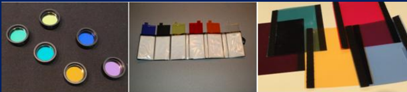
Various Filters and Gels which are used to Examine Playing Cards for Different Daubs & Markings
